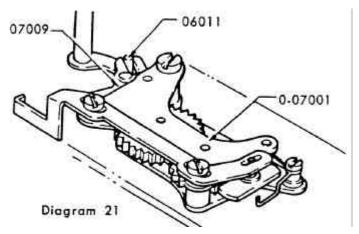
Push the pallet switch lever (07004) in front of the slow speed governor to the right as viewed from the body front. When  $(G\ 04)$  is hit with the pallet release lever bottom (06007), it moves to the right, and the pallet (07003) is separated from the star wheel (07008). At this point, turn (06006) and (06010) clockwise, and the tip of (06006) hits the protruded part of (05057). Pressing down the tip of (06006) onto (05057), fasten it with two set screws  $(Set\ 1.\ 1.4\ x\ 2.5)$ .
