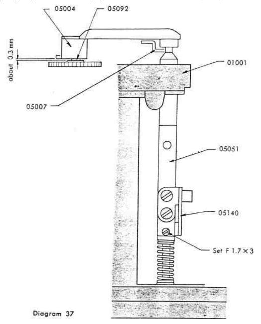
At the instant the mirror seat (02009) flips up, there should be a clearance of approx. 0.3 mm between the under-surface of the release plate (05004) and the upper surface of the collar of the intermediate gear retainer screw (05092). Consequently, (05004) drops farther by approx. 0.3 mm the moment the mirror seat flips up. If the clearance is found excessively bigger or smaller than the limit of 0.3 mm, adjust the shutter actuator plate B (05140) again.
