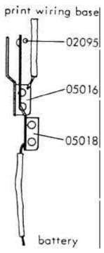
e. Adjust the position of (05016) with tweezers so that it does not touch (05018) when the AM switch lever (01069) is pushed down. (in a state that the switch actuator pin(02095) is moved to the right as shown in Figure 1. d.
