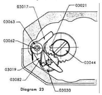
It is important that the two gears engage smoothly. If the gearing of the cogs is unsatisfactory, replace counter dial ratchet with a new one with proper size. For adjusting purposes, counter dial ratchet is available in three different sizes: (03219), (03319) and (03419).
