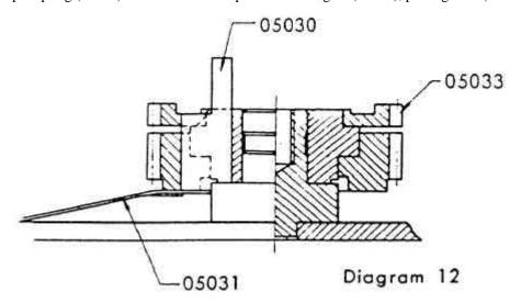
If the groove of (05033), after installation, cannot be properly positioned even though the engaging position of the gear is changed, the groove of (05033) needs adjustment by filing with a fine file.
