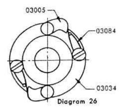
ratchet wheel (03023) with the spring tension. When one tip of (03005) is engaged with (03023), the other tip should be between the cogs of (03023). This permits many sectional cockings for film advance and shutter cocking. See that the outside of (03080) is slightly in contact with the inside of the body proper when the notch "A" at the upper part of (03034) is positioned towards the lever stopper (03004) as illustrated in Diagram 27.
