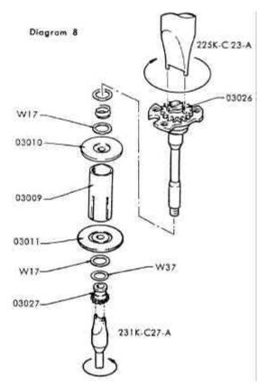
Slightly rotate the top main gear retainer screw (03044) clockwise with a screwdriver, and ease the force of your driver-holding hand, at which determine if the bottom main gear (03026) will revert itself steadily, say, by 2 or 3 cogs of the gear.
