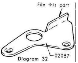
(02085) and dia actuator lever B (02086) in the shaft direction with use of washers. The dia actuator lever A (02085) should be devoid of curvature as the side of the synchro seat (02026) serves as its stopper.
