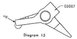
Assemble the high speed lever (0-05005) with the bulb lever (05007), and insert them again into (05050). Hook the high speed lever spring (05120) on the indicator seat (05104) and screw the bulb lever nut (05103) onto (05050). Check with the tip of tweezers if both parts (0-05005 & 05007) move smoothly.
