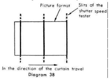
Measure the exposure timing at 1/60 sec. (16.7 ms). Since the bounce of the 1st shutter curtain has not as yet been properly adjusted at this stage, the exposure timing at the end of the picture format is generally registered much faster than at the start or at the centre of the picture format.
