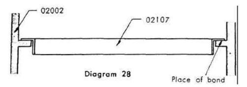
(2) When fixing the mirror seat assembly (0-02009) to the mirror housing (02002), the "A" part of the hinge cover (02011) as shown in the following diagram should not protrude or sink itself from the back of (02002), namely, the "B" part as illustrated in diagram 29, as the shutter curtains may jam with the "A" part. Adjust (02011) correctly with pliers, where required.
