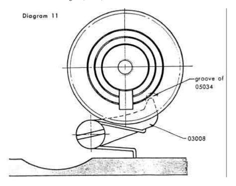
When the force of the screwdriver is eased, the bottom intermediate gear (05034) slightly revolves clockwise with the reversing strength of the wind-up shaft (03042) and stops when it hits the non-return arm (03008).
