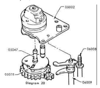
Apply "L-1" lubricant between (06008) and (06009); and between (05002), (05003) and (06002).
