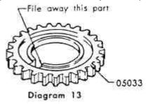
Place the spill recepctacle plate (05032) on the top intermediate gear (05033), and screw the intermediate gear retainer screw (05092-1) onto the intermediate gear shaft (05048).
