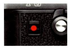
3. Watch the blinking red LED (5) on the front of the camera. The LED blinks faster during the final two seconds before the shutter opens to warn you to get ready.
