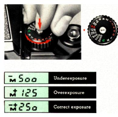
In addition to automatic stepless shutter speed control, the Nikon F3 offers manual control of all shutter speeds from 1/2000 sec. to 8 sec. including X, B, and T. To move the shutter speed dial off "A," depress the locking button 1 as you rotate the dial counterclockwise to the 1/2000 sec. setting. You can then rotate the dial freely
