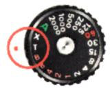
The F3 has two separate settings for time exposures. On "B," the shutter remains open for as long as the shutter release button is depressed. On "T," the shutter stays open until the dial is rotated to another setting, making it ideal for really long time exposures. Being a mechanical setting, "T" will not cause battery drain regardless of how long the shutter remains open.
