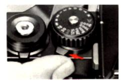
4. Don't forget to return the selt timer to its original position after using it.
