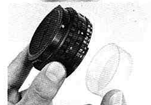
2. Remove the rear lens cap.
