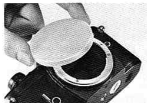
1. Remove the camera body cap.
