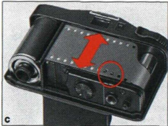
the take-up spool. Push the film leader underneath the metal sleeve as far as it will go (illustration b), then let go of the rewind release button.
