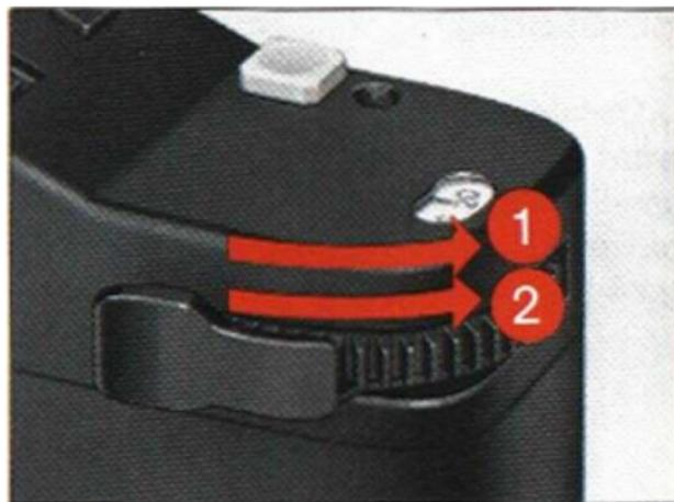
When the whole film is exposed, the transport lever no longer swings out fully and the release is blocked.
