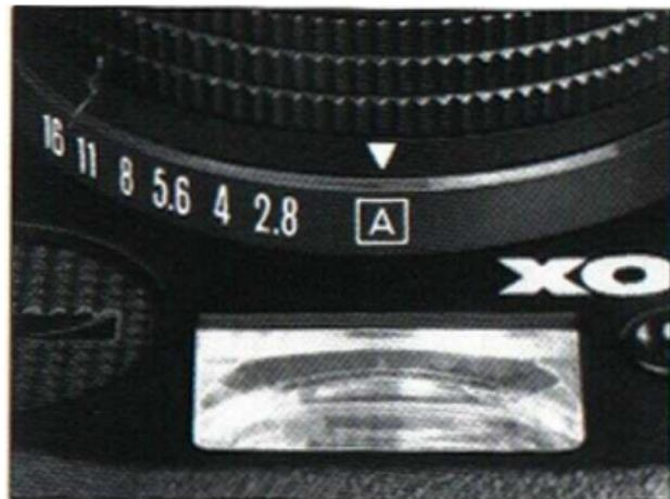
The electronic program of the Minox 35 PL yields aperture/speed combinations from f/16 to f/2.8 and from 1/500 to 4 seconds at 100 ASA (up to 15 seconds at 25 ASA or up to 1 second at 400 ASA).
